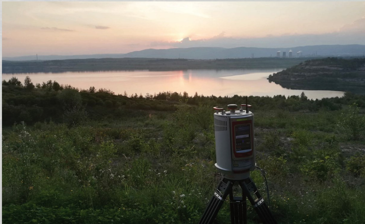
Figure 4 In September 2019, Ineris performed a LiDar 3D survey of the shores of the artificial Most lake. Seventy-five metres deep, this lake was created by flooding an old open-pit lignite mine.
