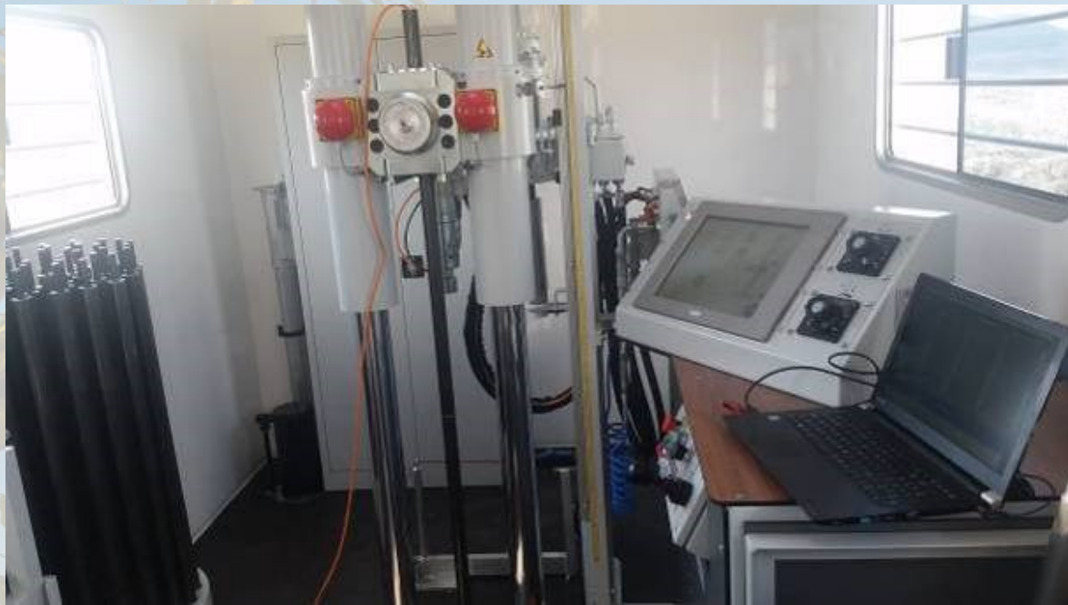
Figure 14 Hydraulic pusher of CPT Unit HYSON-200 kN inside the CPT truck
